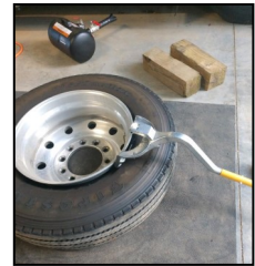
This new tool breaks the bead of the tire from the rim.
